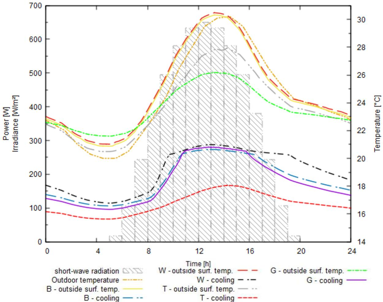
Figure 3: Outdoor temperature at 2 m height and short-wave radiation during the summer scenario, outside wall surface temperatures and power needed for heating in room S for different building scenarios (**B**asic, **W**indows, **T**rees, **G**reen roof and facades)
