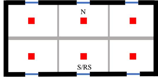
Figure 1: Floor plan of the simulated building. With window positions as small blue lines, heating grid points as red squares, centered north room on 2nd floor N, centered south room on 2nd floor and reference to measurements S, centered south room on 3rd floor under the roof RS.
