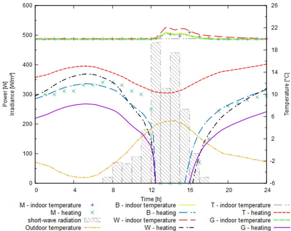
Figure 2: Outdoor temperature at 2 m height and short-wave radiation during the winter scenario, indoor temperatures and power needed for heating in room S for different building scenarios (Basic, big Windows, Trees, Green roof and facades)
