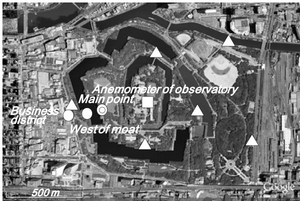
◎: Wind direction and velocity, air, surface and underground temperature △: Wind direction and velocity ○: Air temperature
