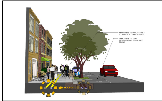
Figure 4. Sample utility core placement diagram for commercial areas
