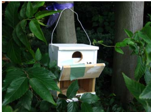
Fig. 6 Sensors installed in birdhouses to measure air temperature and humidity in the premises woods
