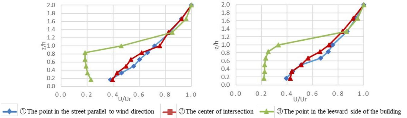
Fig.2 Wind tunnel results of wind velocity with height (Left : prism, Right : cylinder)
