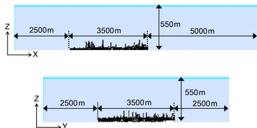
Fig. 3 Cross section of calculation domain in the target area 5-4
