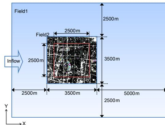
Fig. 2 Plan of calculation domain in the target area 5-4
