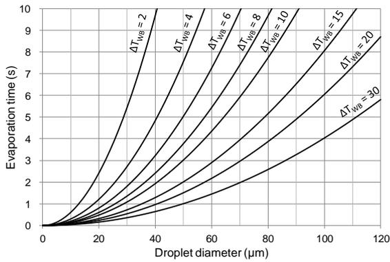
Fig. 4. Time to complete evaporation for single droplets of water in unchanging air conditions.
