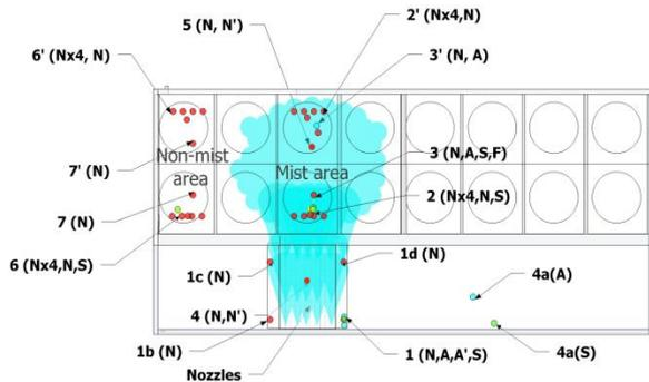
Fig. 8. Layout of the sensors (Top view, locations not to scale)
