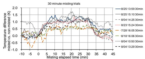
Fig. 13. Temperature differences arising between misted and non-misted areas at outlet during misting.
