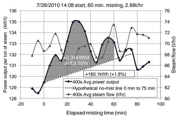
Fig. 14. Example of difference between time-averaged actual power output (solid line) and hypothetical non-misting (dotted line). Area under the curve represents the total power increase.
