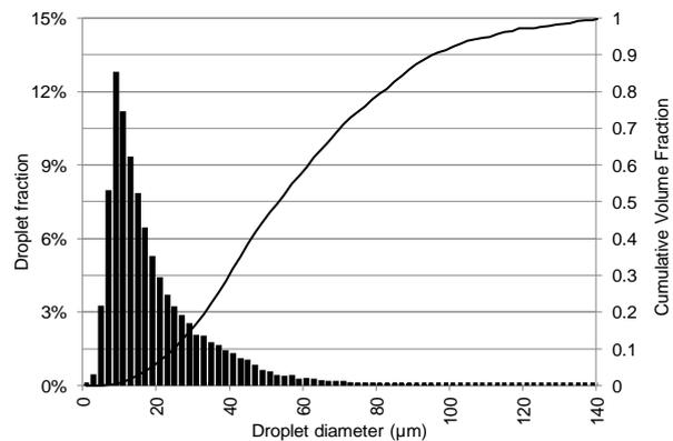
Fig. 6. Nozzle droplet diameter distribution (in 2 µm bins) and cumulative volume fraction.
