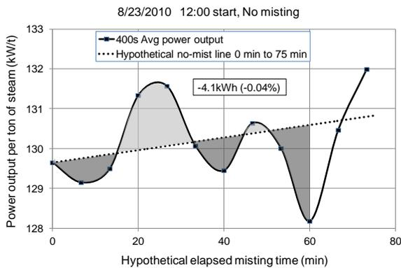
Fig. 15. Example of check for bias using the integration method for a period without misting.
