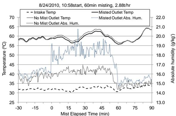
Fig. 12. Example case of temperature and abs. humidity above condenser in the misted area and no-mist area during a 60-minute trial.
