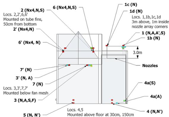
Fig. 9. Layout of the sensors (Side view, locations not to scale)
