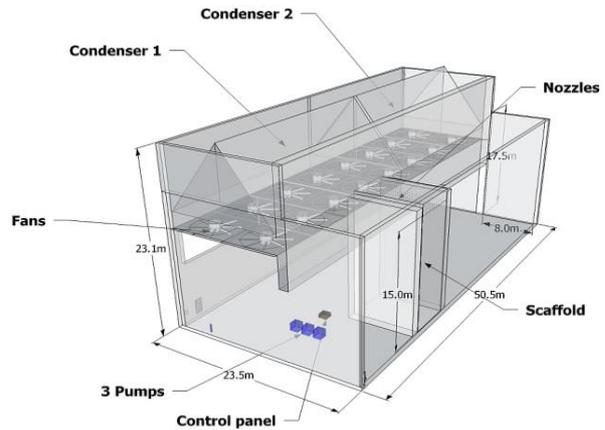
Fig. 5. Layout of the condensers, air inlet section, and installed misting system.
