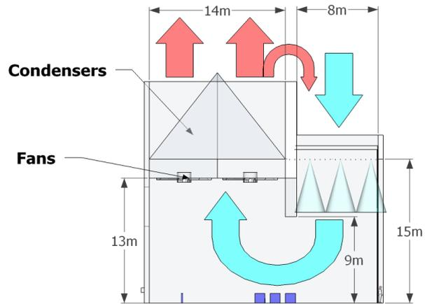
Fig. 7. Cross-section of plant condenser area and nozzle position. Arrows indicate flow of air and mist.
