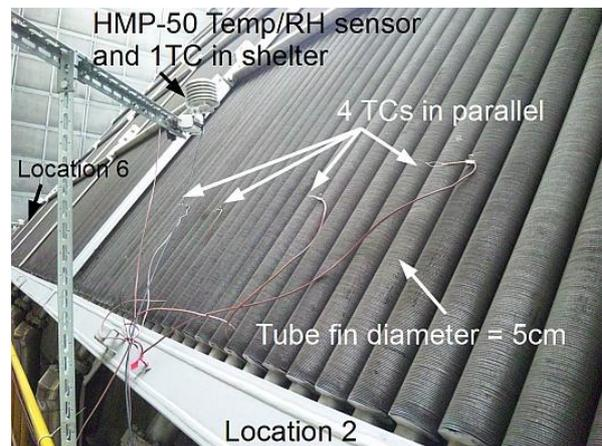
Photo 2. Sensors at Location 2. Thermocouples (TCs) in parallel to average out local differences among fin tube temperatures. Location 6 visible in background at left.
