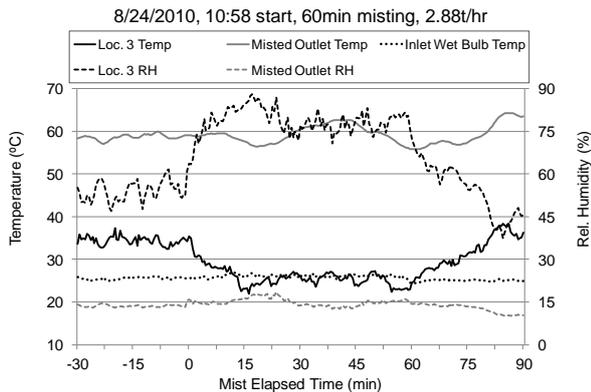
Fig. 11. Temperature and Rel. Humidity in the misted area at the outlet (Loc. 7) and below the condenser fans (Loc. 3) where sensor wetting clearly occurred.
